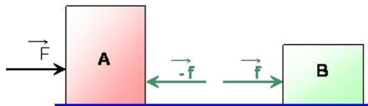
$$\begin{aligned} F_R^A &= M_A \cdot \alpha \\ F - f &= M_A \cdot \alpha \\ 20 - f &= 2 \alpha \end{aligned}$$
